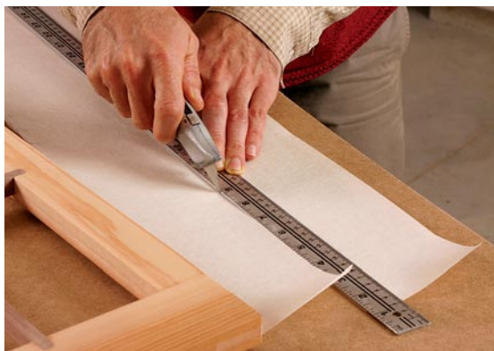
Cut the paper to size. A long rule and a sharp utility knife are all that is needed to cut the paper.
