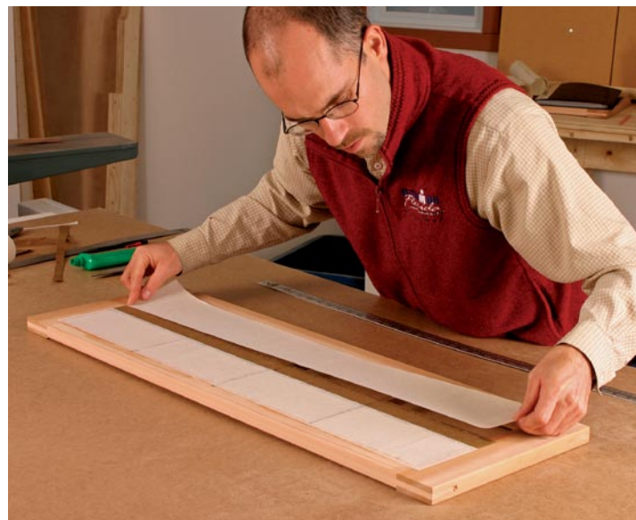
Keep the paper parallel. It is easy to misalign a long piece of paper, so line it up with the frame or a divider before pressing it down.
